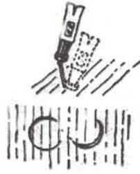
Strike nail squarely to avoid bending nail and denting the wood.
