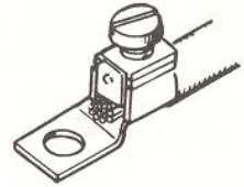
Solderless connectors of this type are used with heavy sizes of wire.
